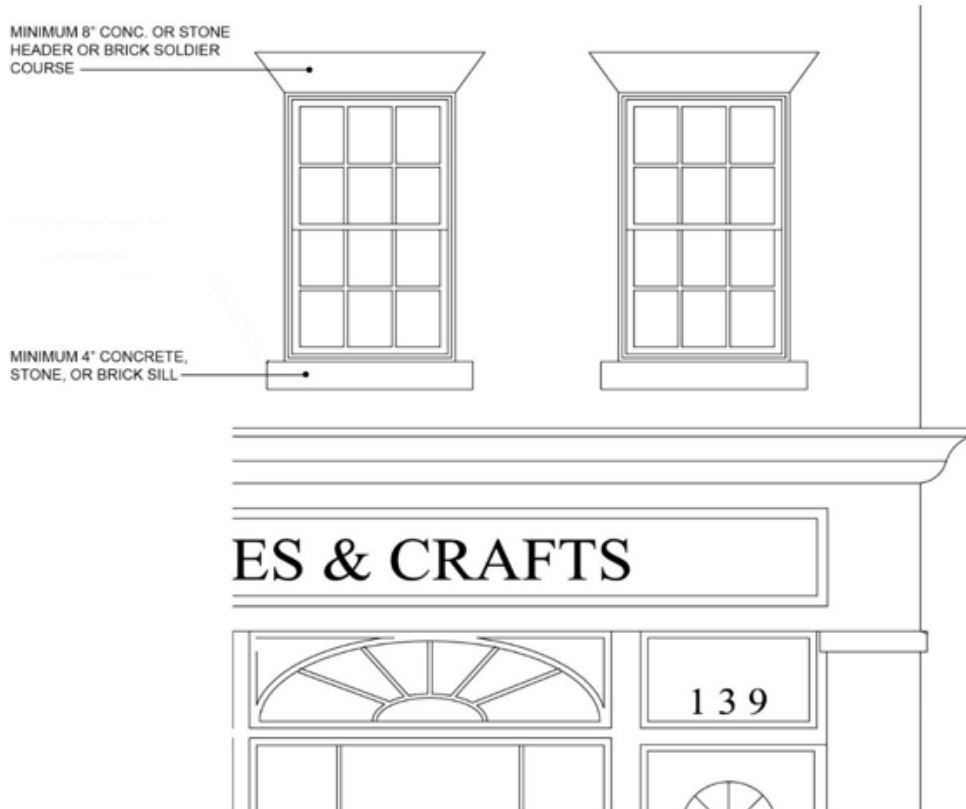
Figure 2.10: Treatment of Masonry Windows
